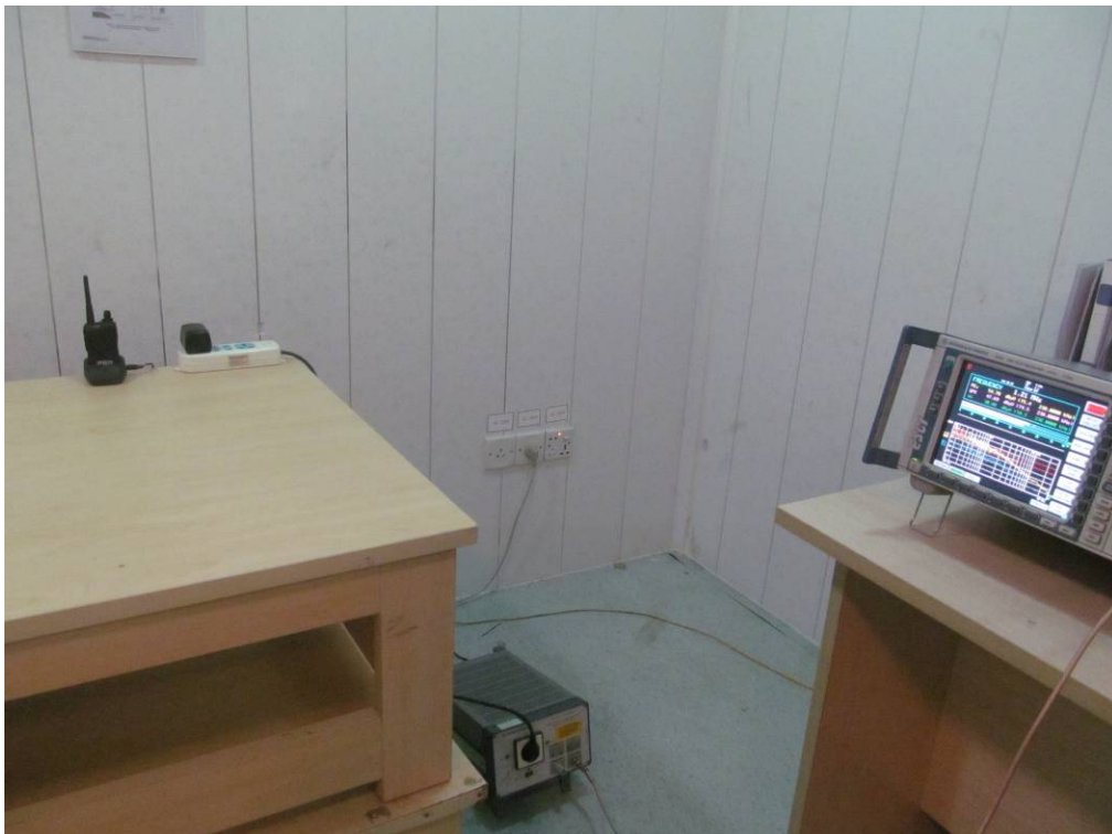
CONDUCTED EMISSION TEST SETUP
