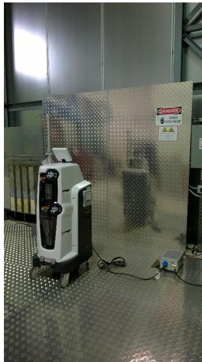
Figure 3.6-2: AC Powerline Conducted Emissions Setup
