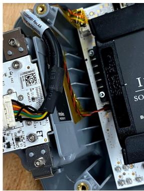
NFC Antenna Mounted and Connected to PCBA
