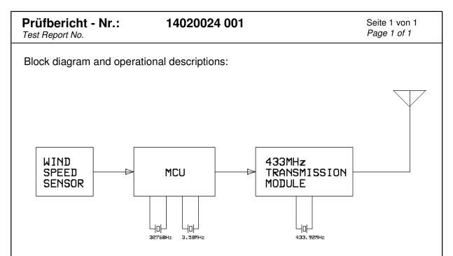
TS815 is a wind speed transmitter which can measure wind speed and transmit a wind speed signal. While detect a wind from the wind impeller, the wind speed signal will convert to an electronics signal through Q10 to MCU. After the analysis of the wind speed by MCU, it will transmit the wind speed signal through a 433MHz transmitting module with 33 seconds interval.
