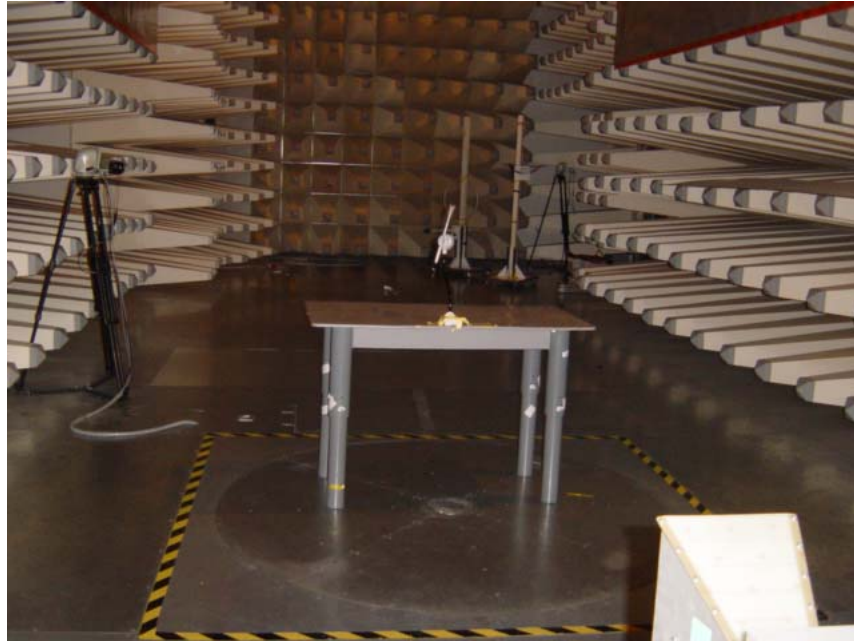
Set up of radiated emission test
