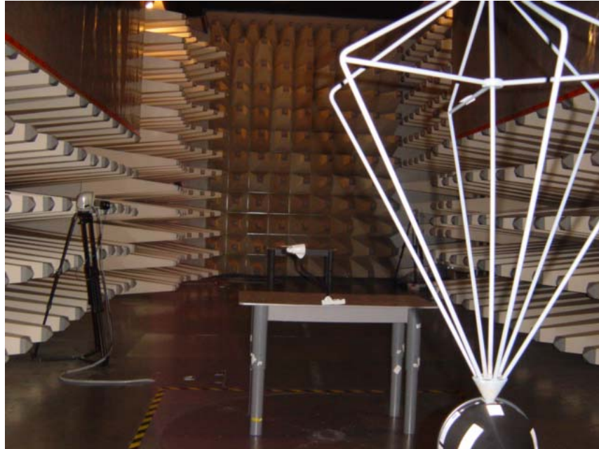
Set up of radiated emission test
