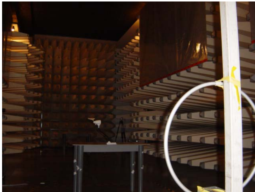
Set up of radiated emission test
