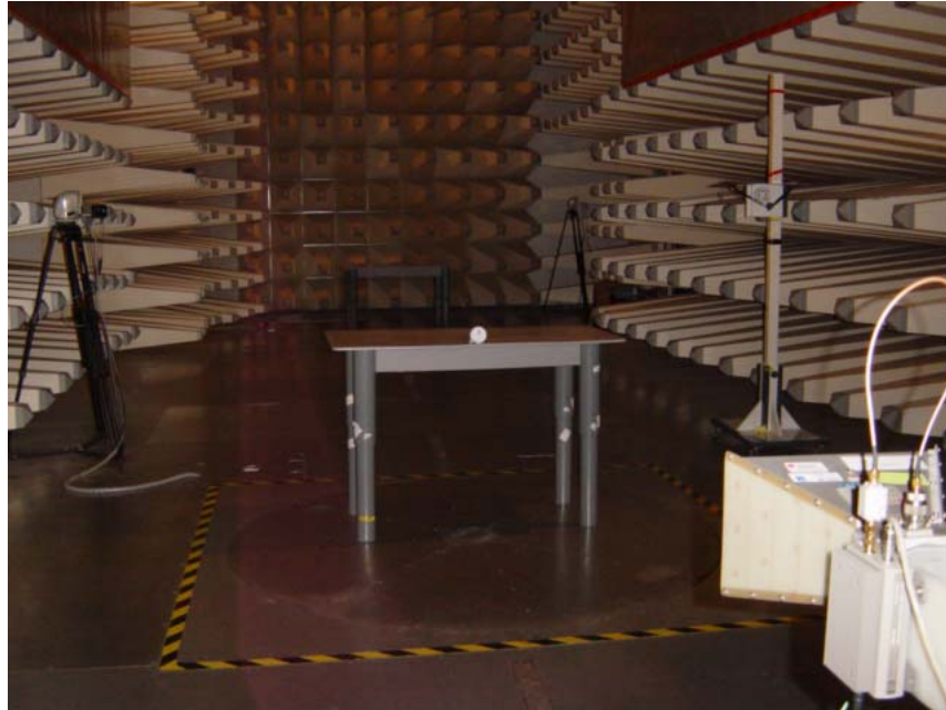
Set up of radiated emission test
