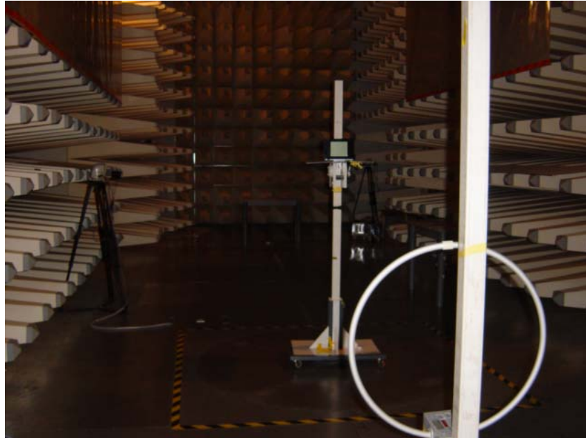
Set up of Radiated Emission Test
