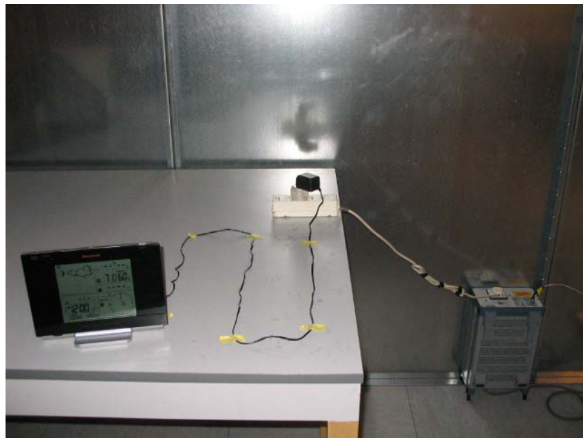
Set up of Conducted Emission Test
