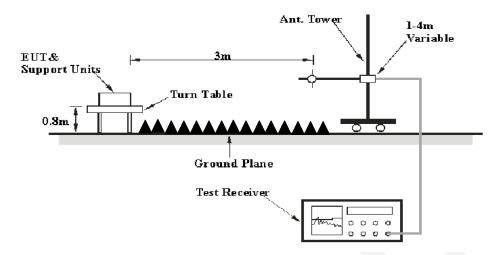
The radiated emission tests were performed in the 3 meters chamber test site, using the setup accordance with the ANSI C63.4-2003. The specification used was the FCC Part 15.109 Class B limits.
