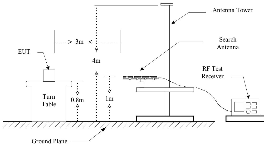
Figure 2 : Frequencies measured above 1 GHz configuration
