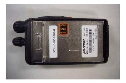
The consumer packaging for these models includes the battery pack as a separate item, NOT installed on the radio. As such, the FCC identifier will be readily visible to the user before the battery pack is installed and whenever the battery pack is removed or replaced. In this location, the label will also be protected from physical abuse and remain readable for the anticipated life of the device.
