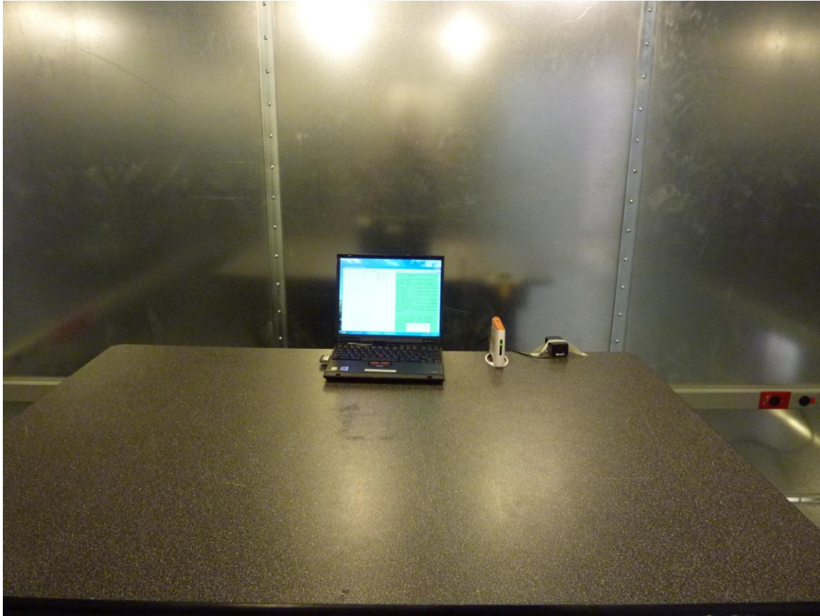
Figure 10: AC Conducted Emission Test Setup for RAP-3WN (Front View)
