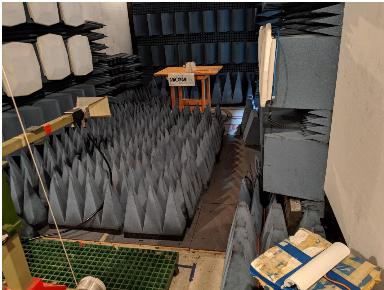
Radiated DFS Test Setup
