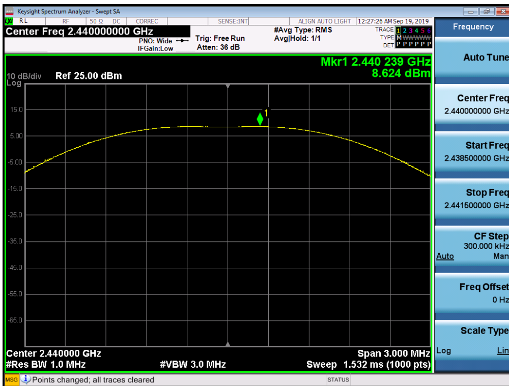
Conducted Output Power (Mid-CH 19)
