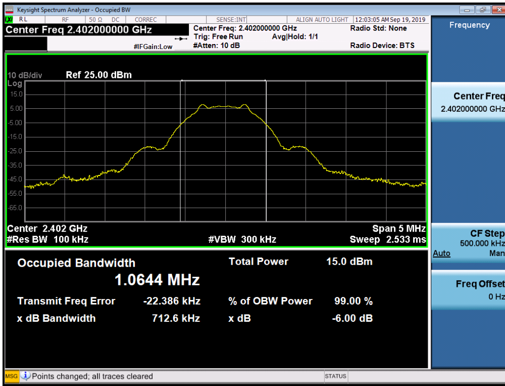
6 dB Bandwidth plot (Mid-CH 19)
