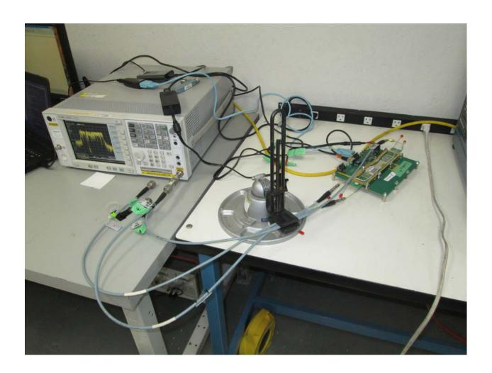
Conducted Emissions Test Configuration Photographs
