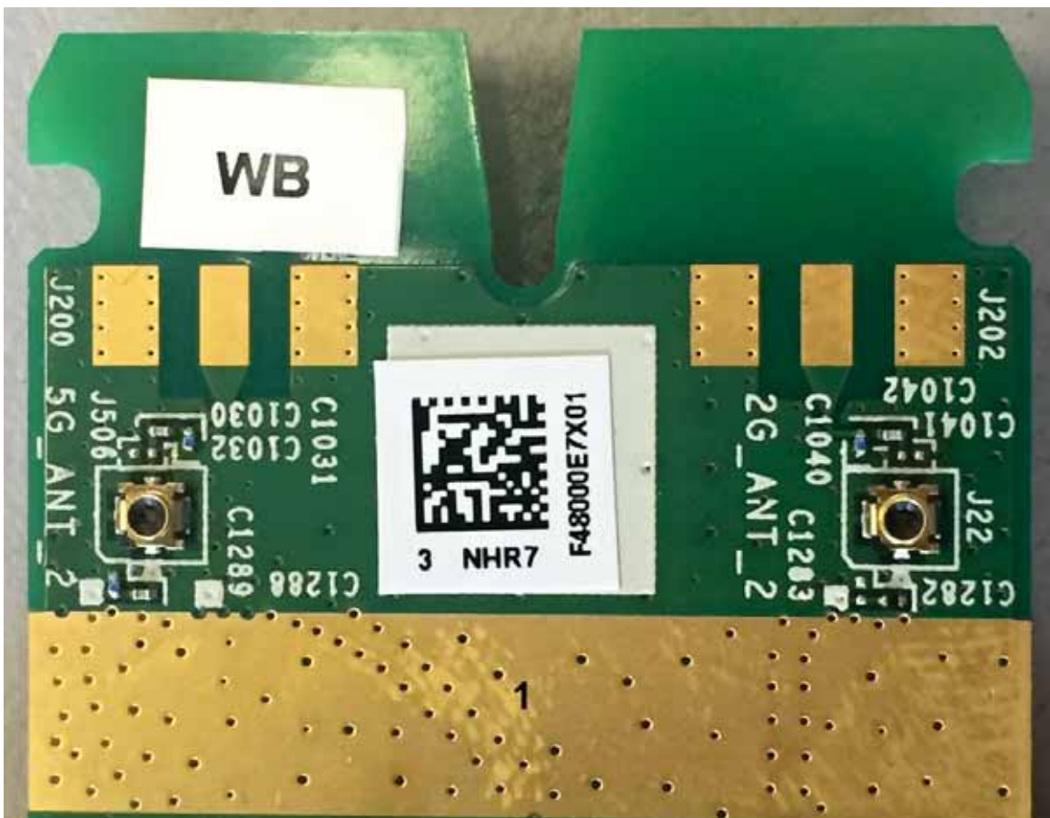
Close-up of Bottom Section Marked 1 - Antenna Ports
