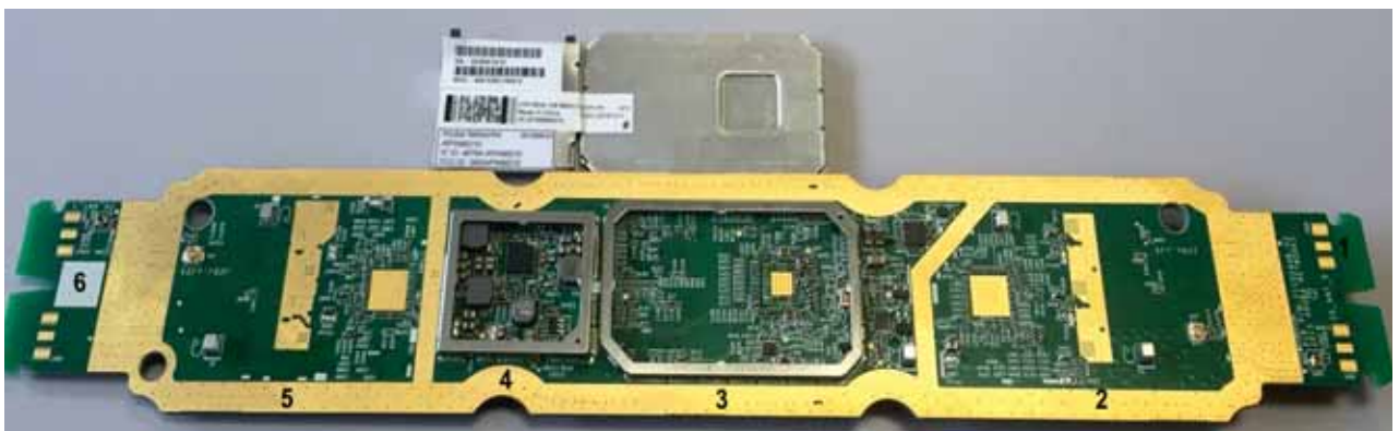
Top View of Module with Shields Removed
