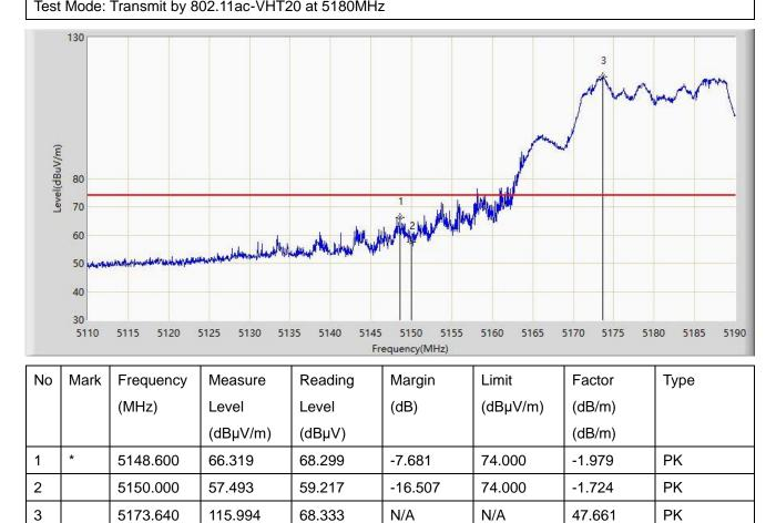
Note 2: Measure Level (dBµV/m) = Reading Level (dBµV) + Factor (dB/m).
