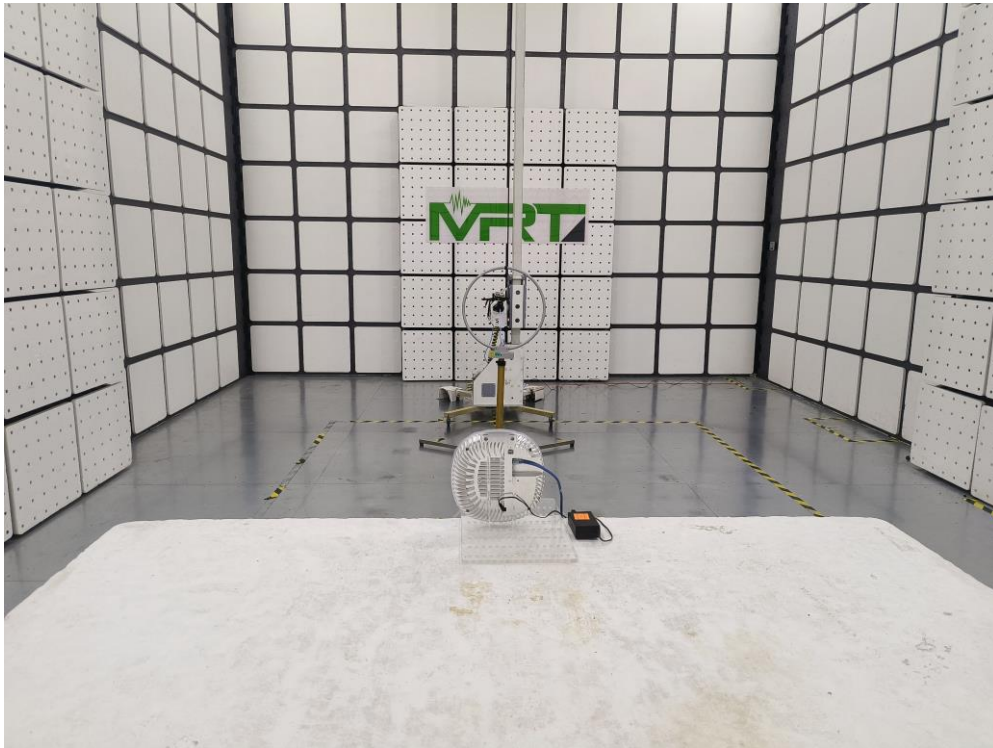
Description: Radiated Spurious Emission Test Setup for 30MHz ~ 1GHz
