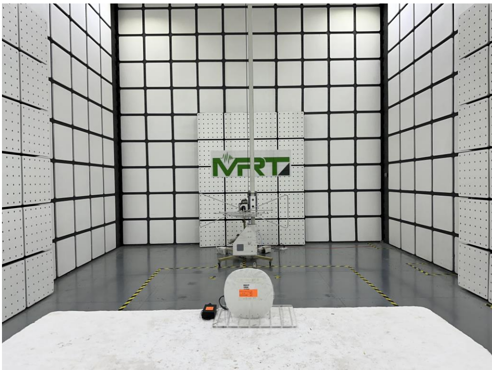
Description: Radiated Spurious Emission Test Setup for 30MHz ~ 1GHz
