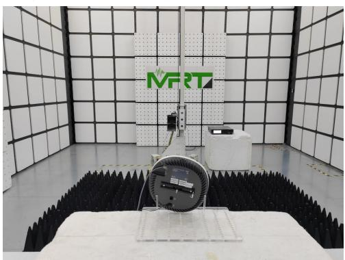
Description: DFS Radiated Test Setup
