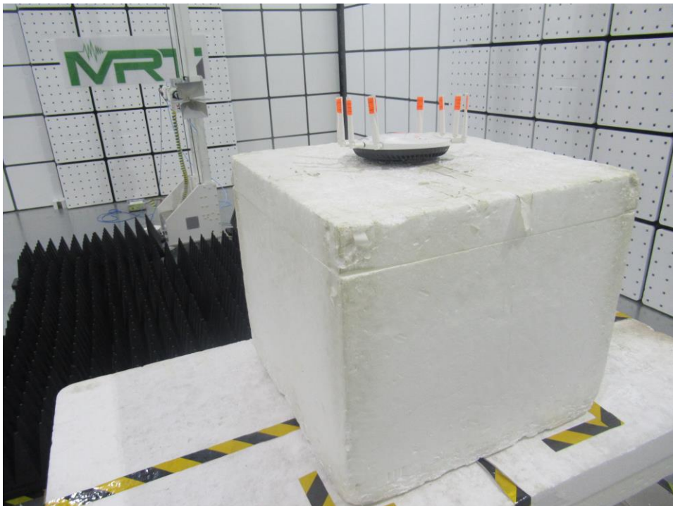
Description: Radiated Spurious Emission Test Setup for Above 1GHz AP-ANT-311
