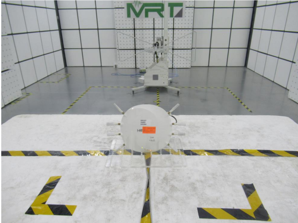
Description: Radiated Spurious Emission Test Setup for Above 1GHz AP-ANT-312
