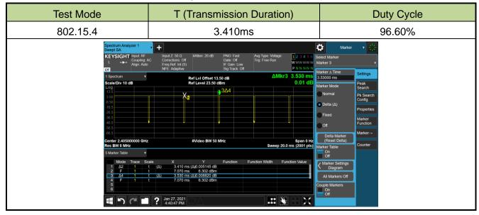
Note 1: This duty cycle was only suitable for continuous transmission of signals via commands. Note 2: The manufacturer, declared that the ZigBee operation, when implemented, will be limited to a max duty cycle of 10% or less in any 100ms period. So -20dB correction factor was used during peak and average band edge testing.
