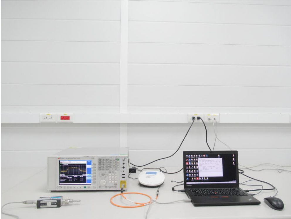
Description: DFS Test Setup _ Conducted
