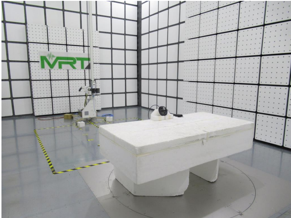
Description: DFS Test Setup _ Radiated
