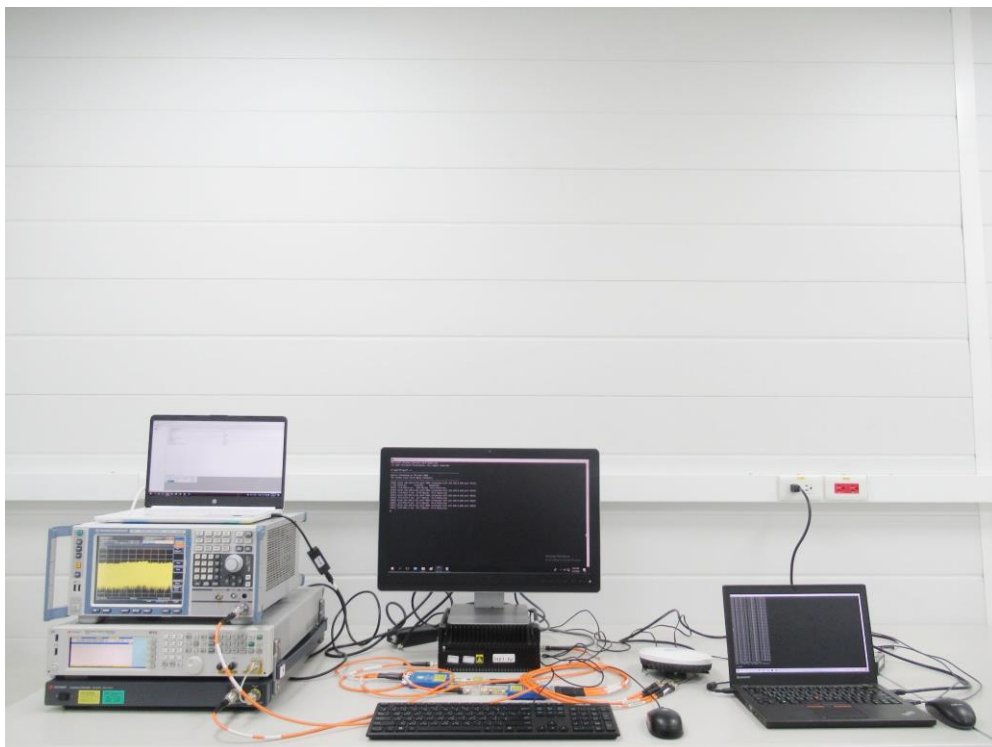
Description: DFS Test Setup _ Conducted
