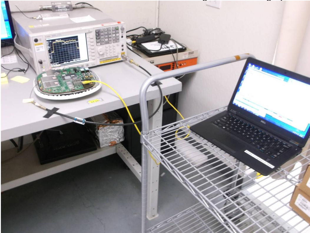
Antenna Conducted Emissions Test Configuration Photographs
