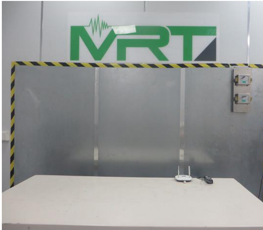
Description: Back View of Conducted Emission Test Setup - APIN0504
