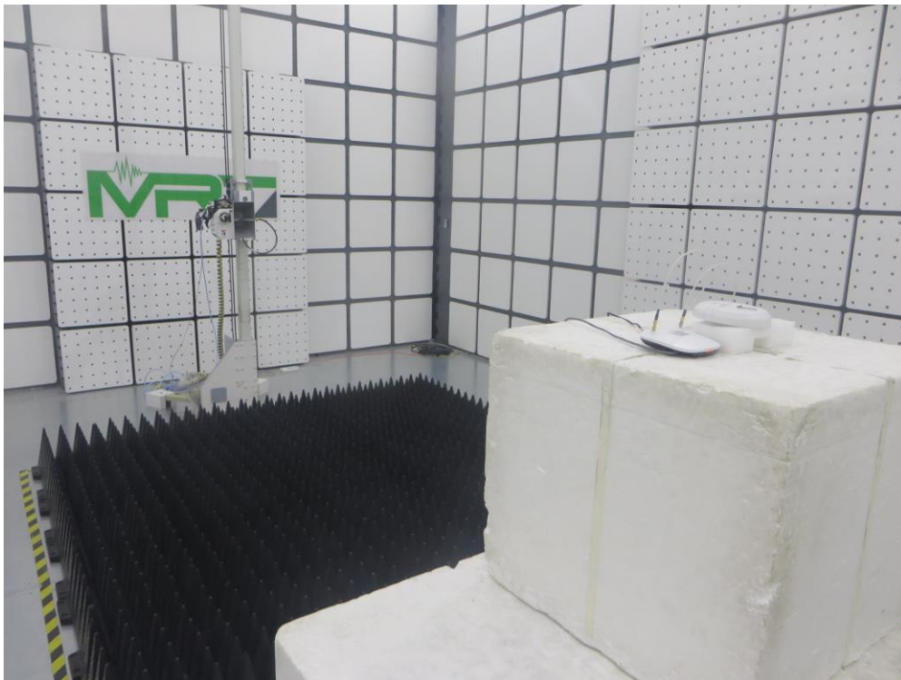
Description: Radiated Spurious Emission Test Setup for Above 1GHz (APIN0504 Antenna: AP-ANT-40)
