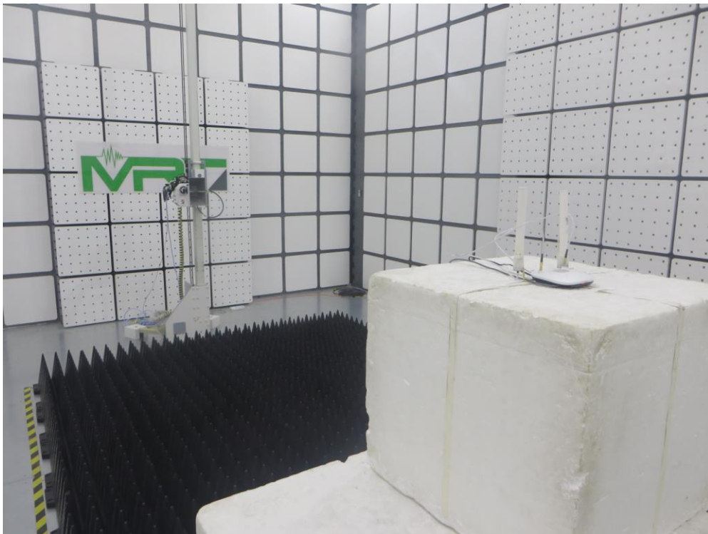
Description: Radiated Spurious Emission Test Setup for Above 1GHz (APIN0504 Antenna: AP-ANT-19)
