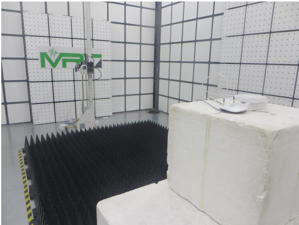
Description: Radiated Spurious Emission Test Setup for Above 1GHz (APIN0504 Antenna: AP-ANT-28)
