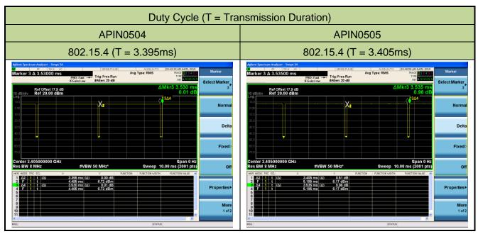
Note 1: This duty cycle was only suitable for continuous transmission of signals via commands. Note 2: The manufacturer, declared that the ZigBee operation, when implemented, will be limited to a duty cycle of 10% or less in any 100ms period. So -20dB correction factor was used during peak and average band edge testing.
