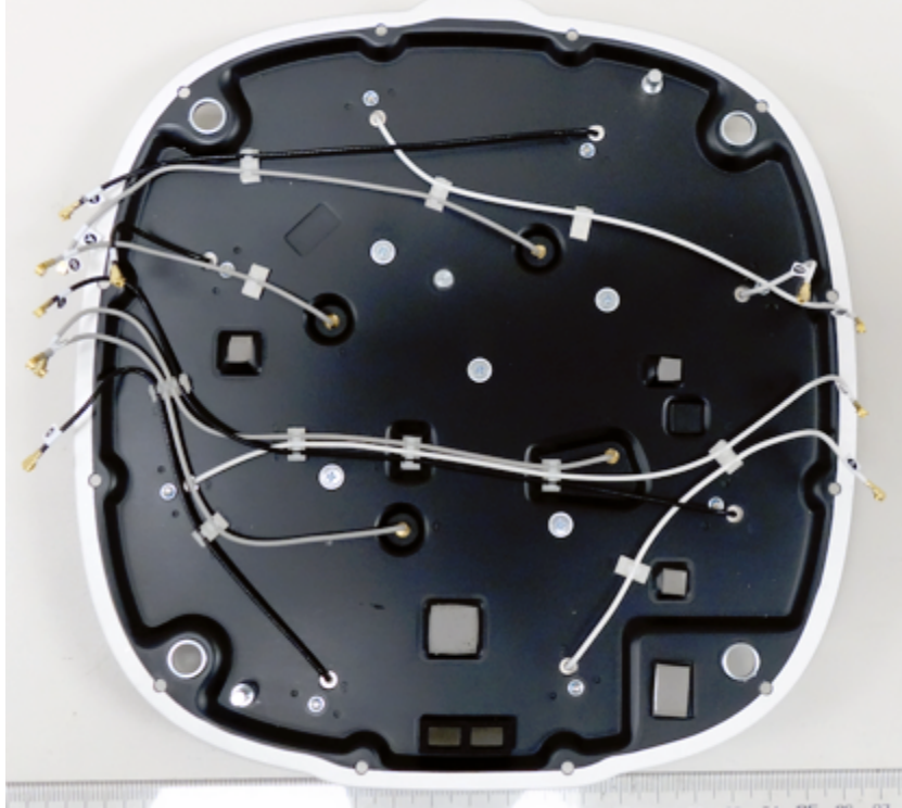
Bottom View of Antenna Plate
