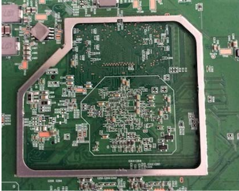
Close Up Main Board CPU Shield Removed
