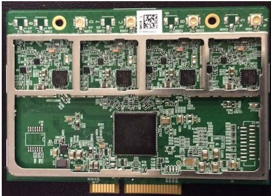
AP325 5GHz Card (Top – Shield Removed)
