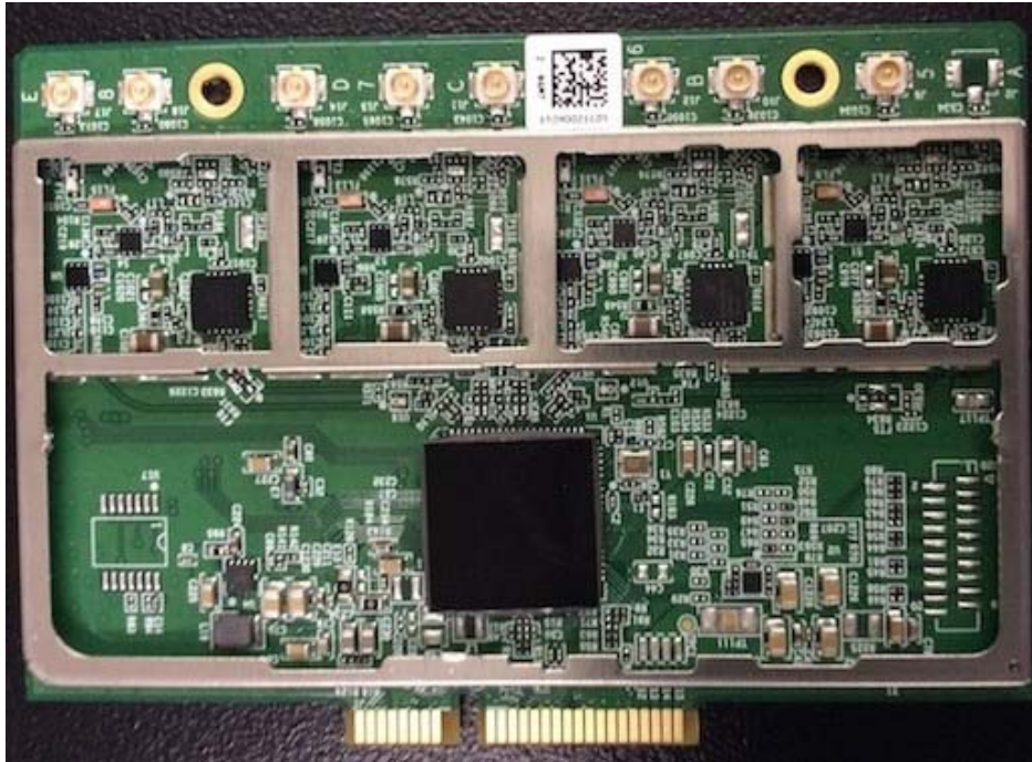
AP324 5GHz Card (Shield Removed)
