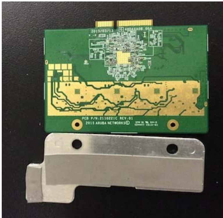
AP325 5GHz Card (Bottom-Plate Removed)
