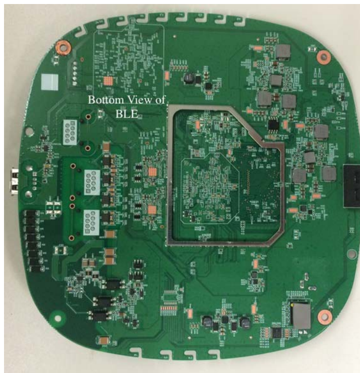
Main Board with Shield Removed (BLE section Labeled)
