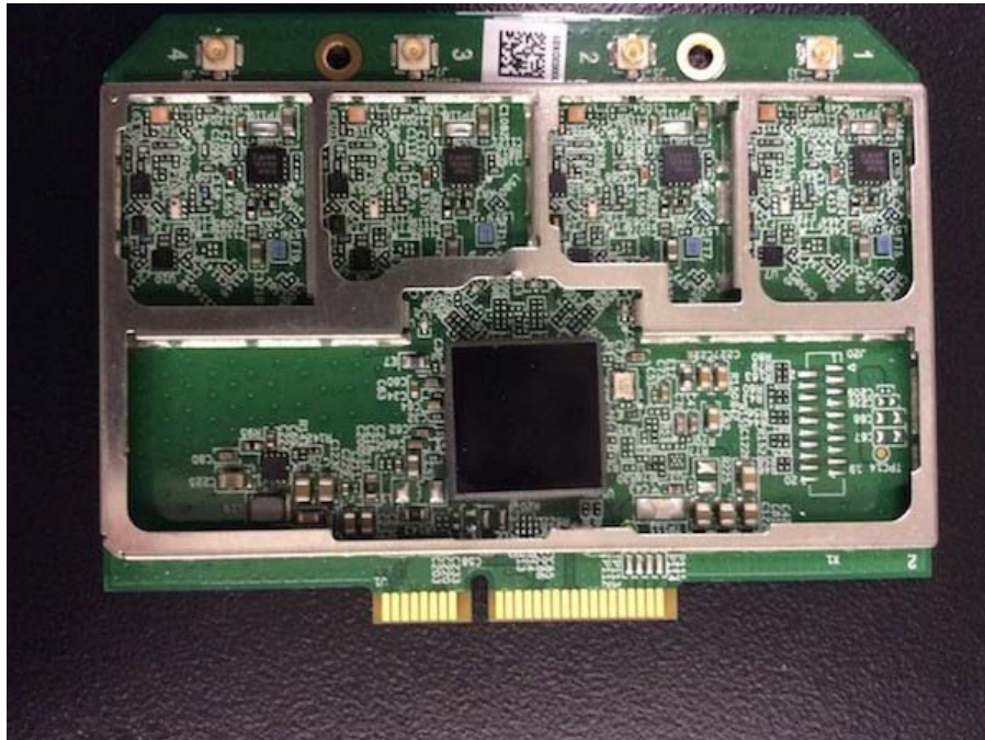
2.4GHz Card (Top-Shield Removed)
