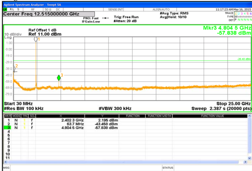
Figure 8: Out of Band Emission for at 2402 MHz
