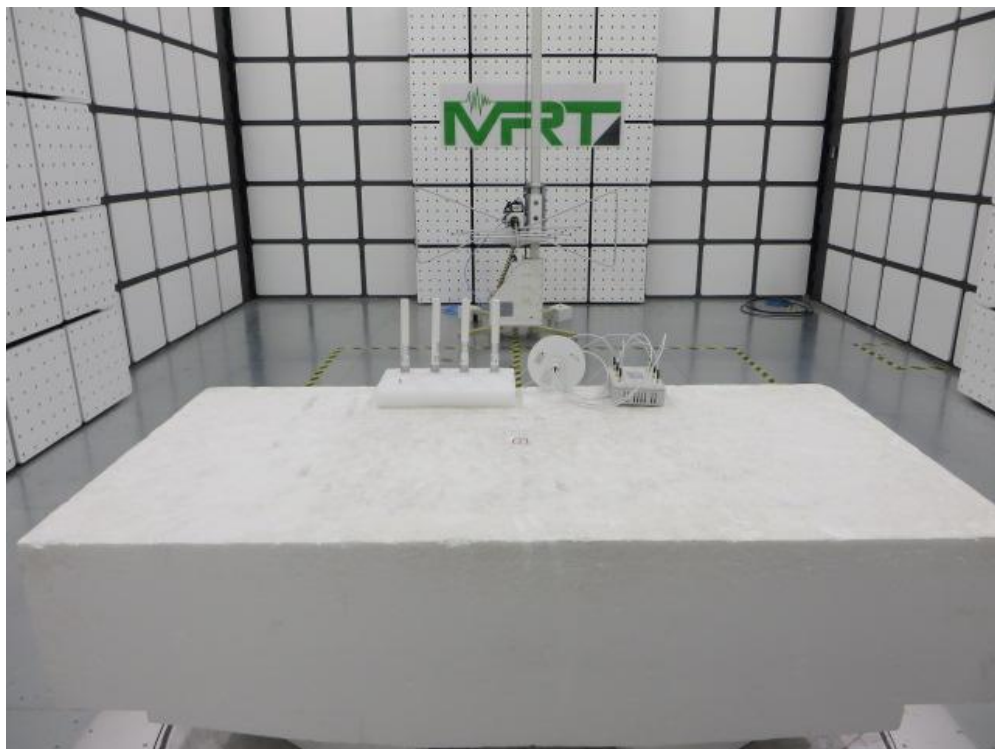
Description: Radiated Spurious Emission Test Setup for 30MHz ~ 1GHz (AP-ANT-19 + AP-ANT-40)
