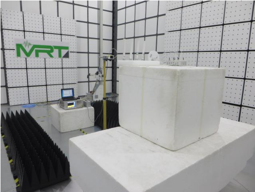
Description: Radiated Spurious Emission Test Setup for 18GHz ~ 40GHz (AP-ANT-19 + AP-ANT-40)
