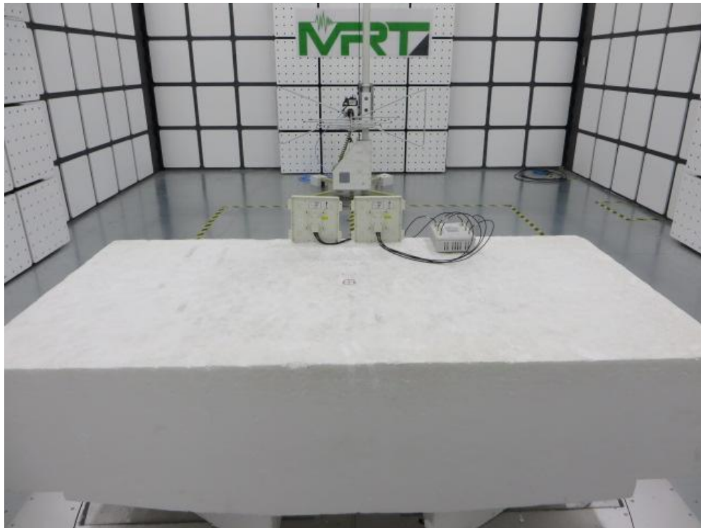
Description: Radiated Spurious Emission Test Setup for 30MHz ~ 1GHz (AP-ANT-48)
