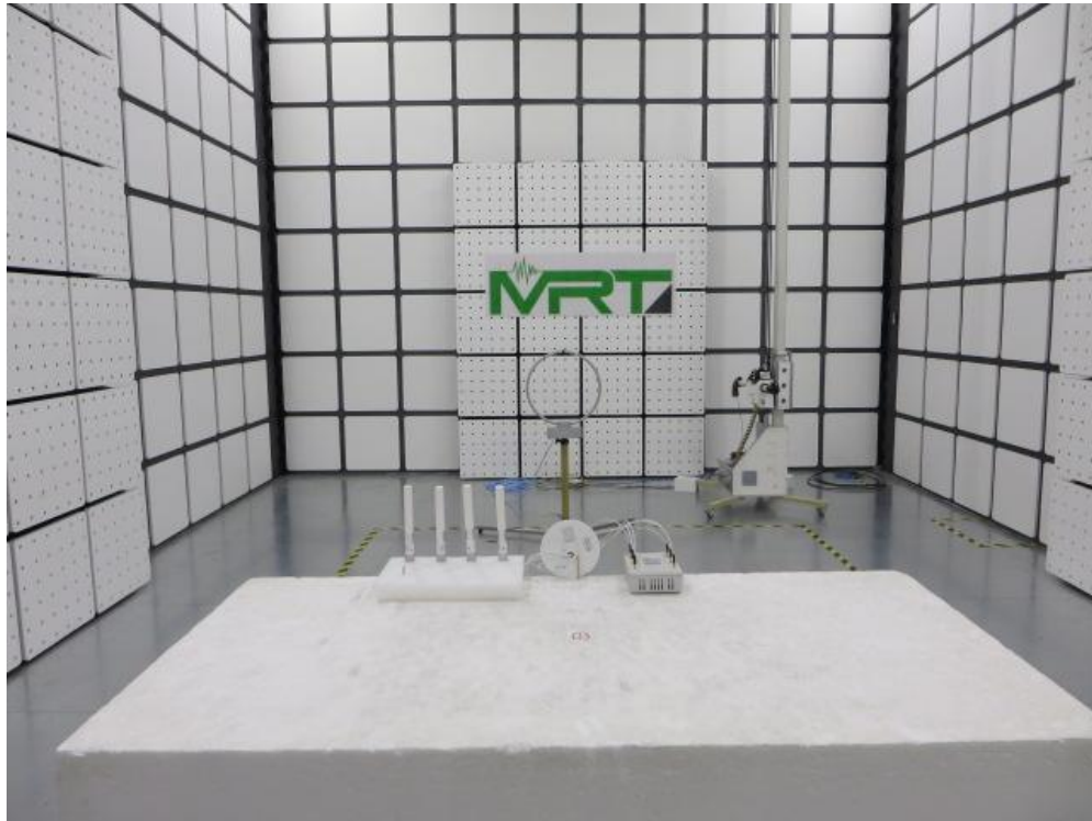
Description: Radiated Spurious Emission Test Setup for 30MHz ~ 1GHz (AP-ANT-19 + AP-ANT-40)
