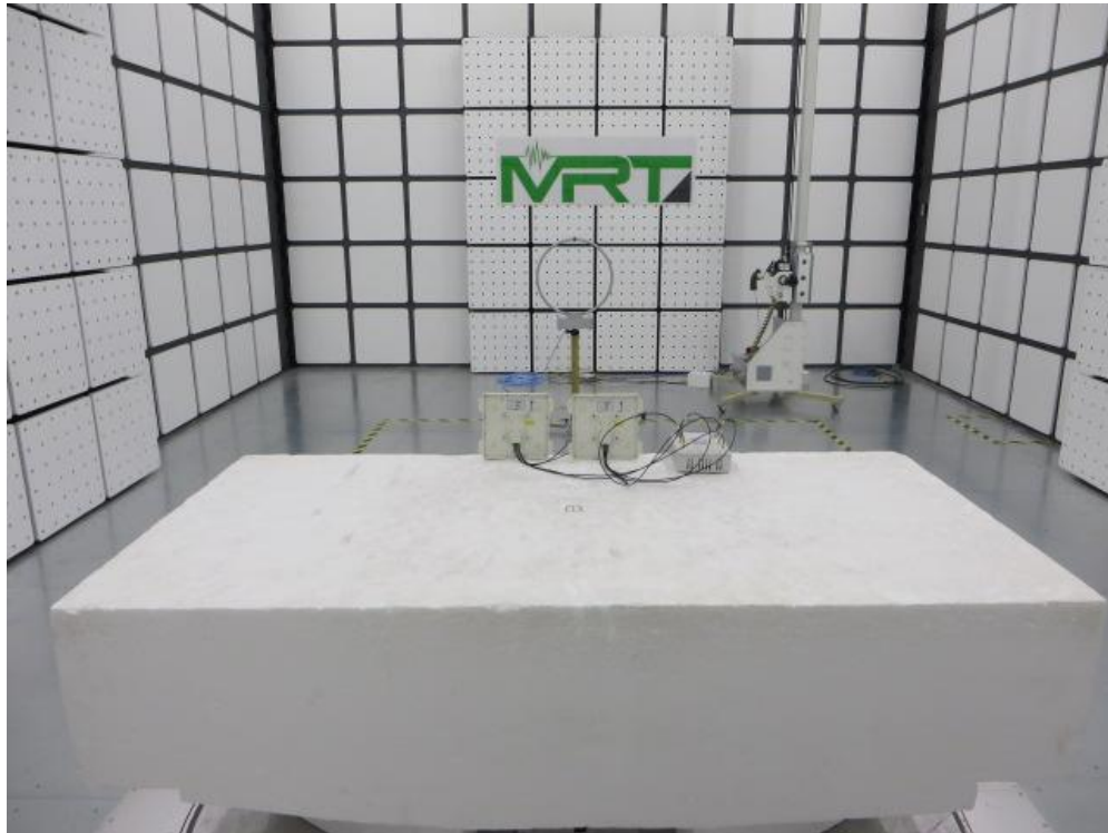
Description: Radiated Spurious Emission Test Setup for 30MHz ~ 1GHz (AP-ANT-48)
