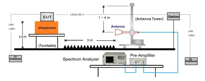
Make the EUT connect with the station by 2.4GHz wireless.
