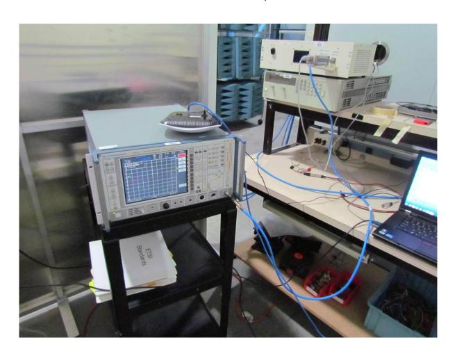
Test Setup - Digital Emissions > 1 GHz
