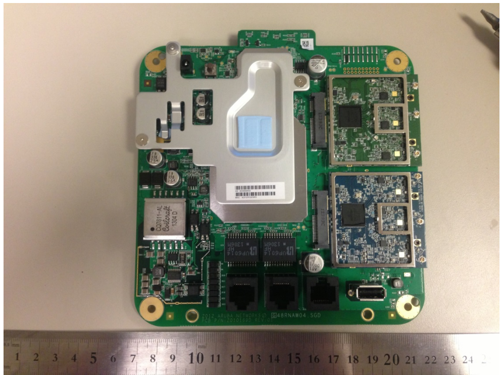
Photo 4– Main Board front View (Radio Cards Shielding off)
