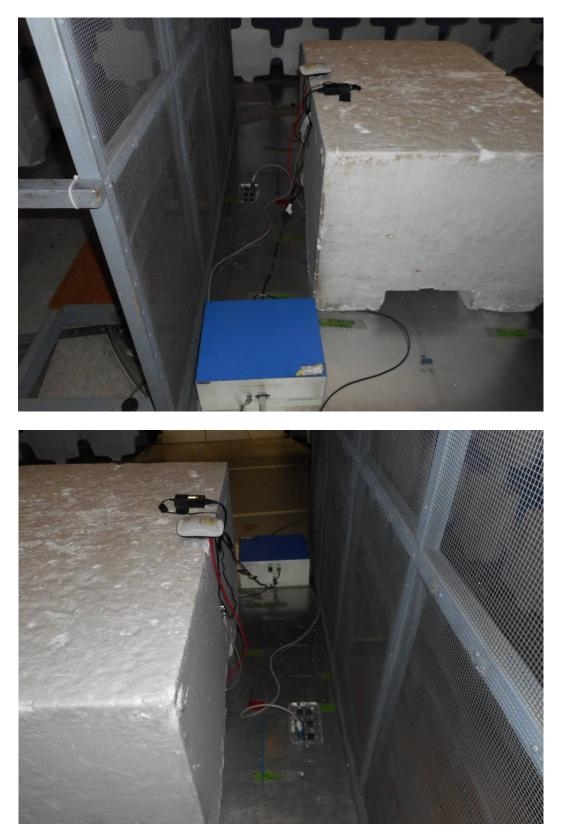
Conducted Emissions Test Configuration Photographs
