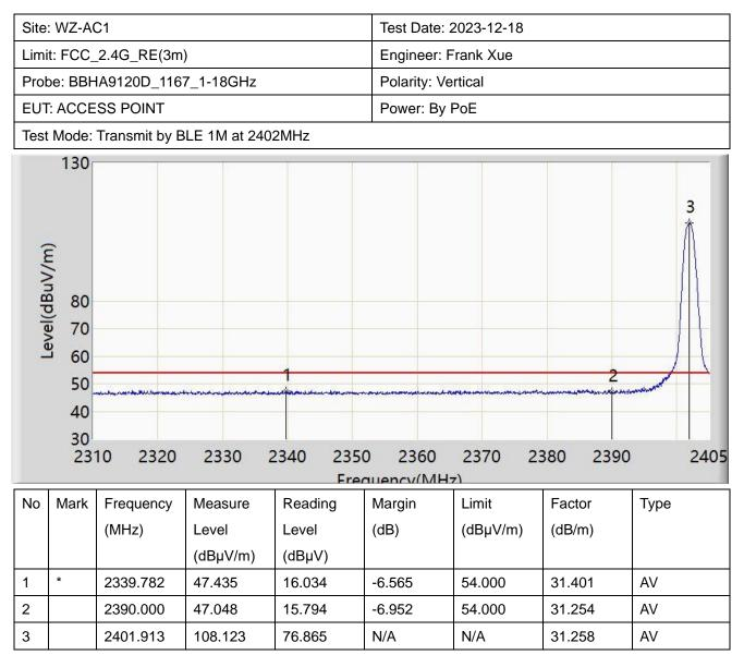
Note 2: Measure Level  $(dB\mu V/m)$  = Reading Level  $(dB\mu V)$  + Factor (dB/m).
