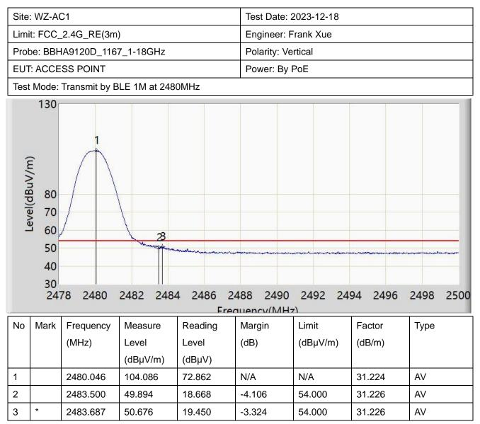
Note 2: Measure Level  $(dB\mu V/m)$  = Reading Level  $(dB\mu V)$  + Factor (dB/m).
