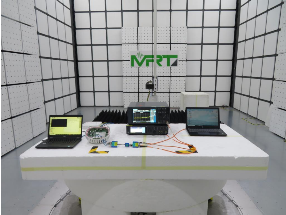
Description: DFS Radiated Test Setup
