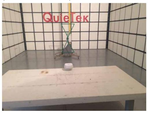
Description: Radiated Emission Test Setup for 1~18GHz
