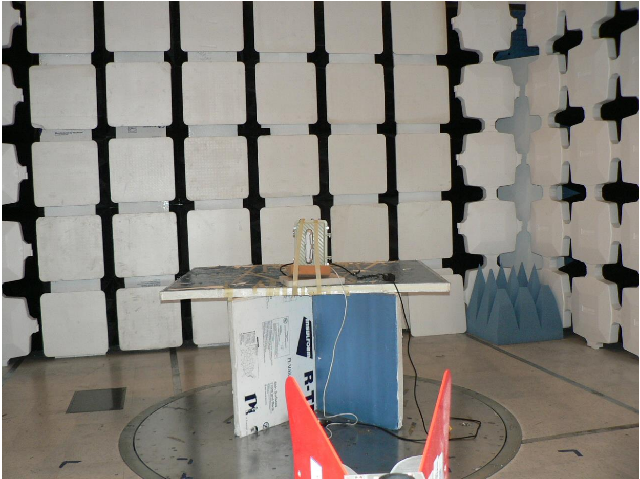
Test Setup - RE#1 - Radiated Emissions - 3m Chamber
