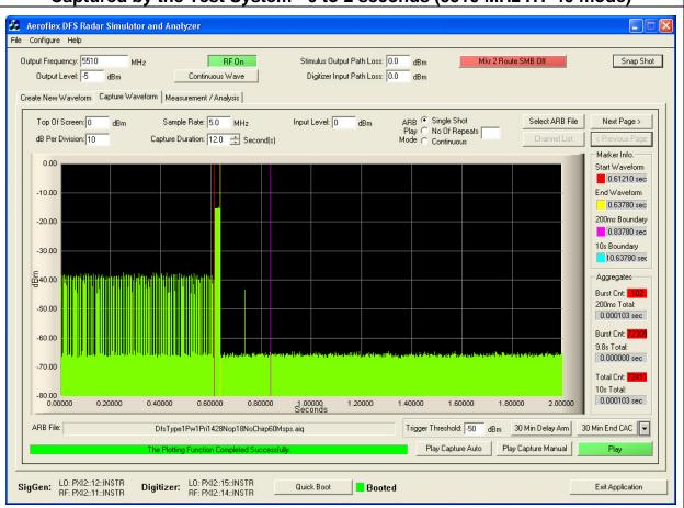
From the plot above it can be seen that the transmission activity within the 200 mS window is 0.103 mS (see 200 mS Total). From the following plots which shows all additional activity within the remainder of the 10 sec measurement window it can be determined that the aggregate transmission is 0.000 mS. This is less than the 60 mS limit.
