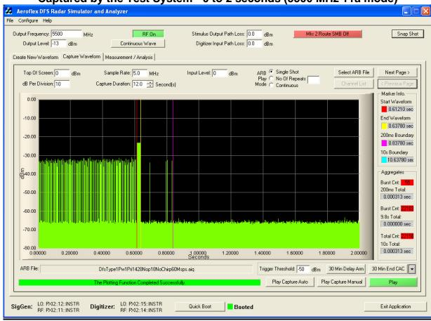
From the plot above it can be seen that the transmission activity within the 200 mS window is 0.313 mS (see 200 mS Total). From the following plots which shows all additional activity within the remainder of the 10 sec measurement window it can be determined that the aggregate transmission is 0.000 mS. This is less than the 60 mS limit.
