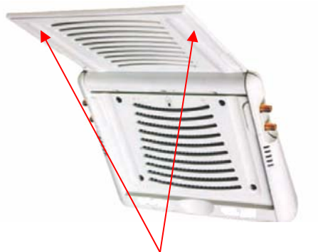
Figure 1: Integrated Articulating Antennas
