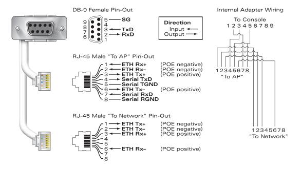
FIGURE B-2 Aruba Serial Breakout Adapter
