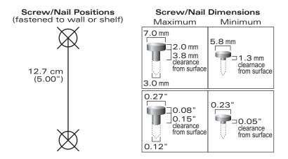
FIGURE 2-3 Mounting Screw Specifications
