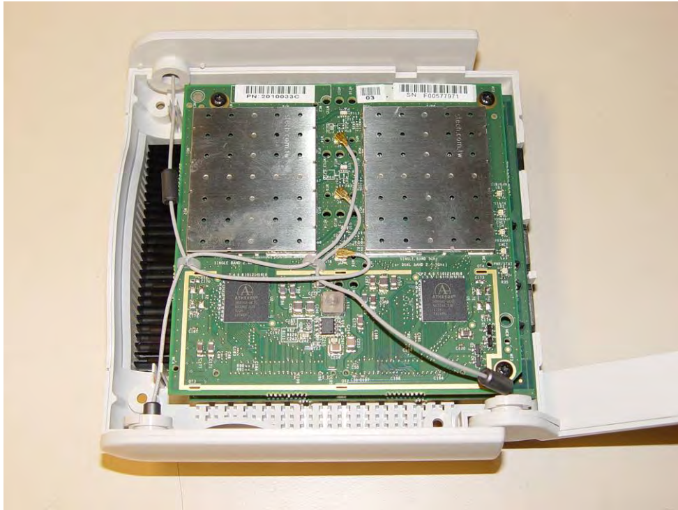
AP125 Internal View
