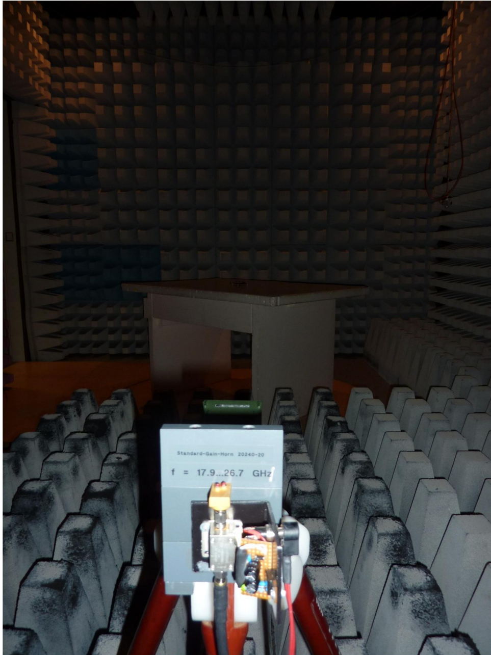
124226_10.JPG: Test setup fully anechoic chamber
