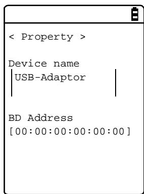
Press the **[F1]** key to display the device name and BD address of the remote device being selected.
