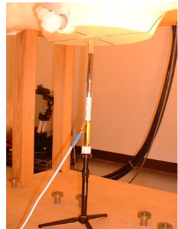
2450MHz System performance check setup
