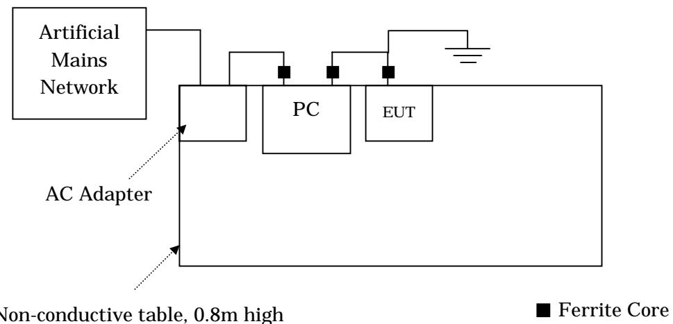
Note : : USB cable was out of the shield and connected to earth line, and EUT was placed on the GND.
