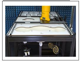
The device holder positions are adjusted to the standard measurement positions in the three sections. A cover is provided to tap the phantom during off-periods to prevent water evaporation and changes in the liquid parameters. On the phantom top, three reference markers are provided to identify the phantom position with respect to the robot.
