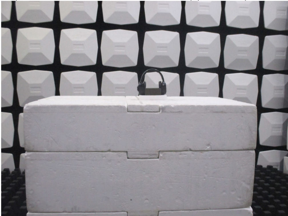
Description: Back View of Radiated Emission Test Setup (Above 1 GHz)
