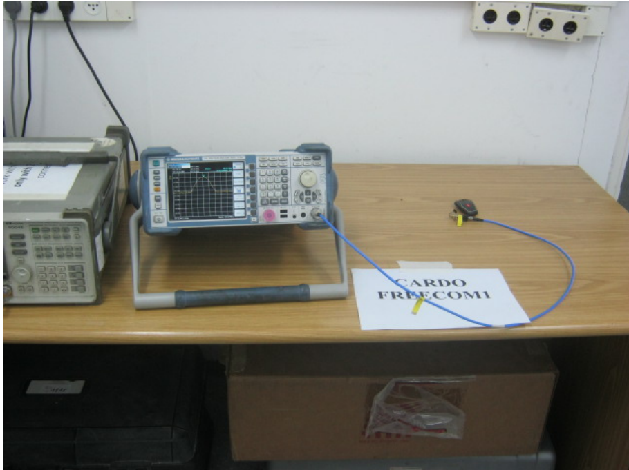
Figure 5. Conducted Emission From Antenna Ports Test Set-Up
