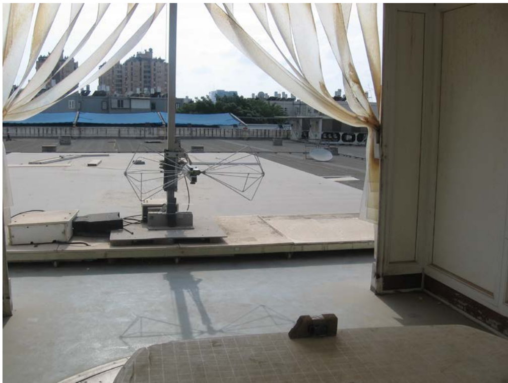
Figure 5. Radiated Emission Test, 30-200MHz
