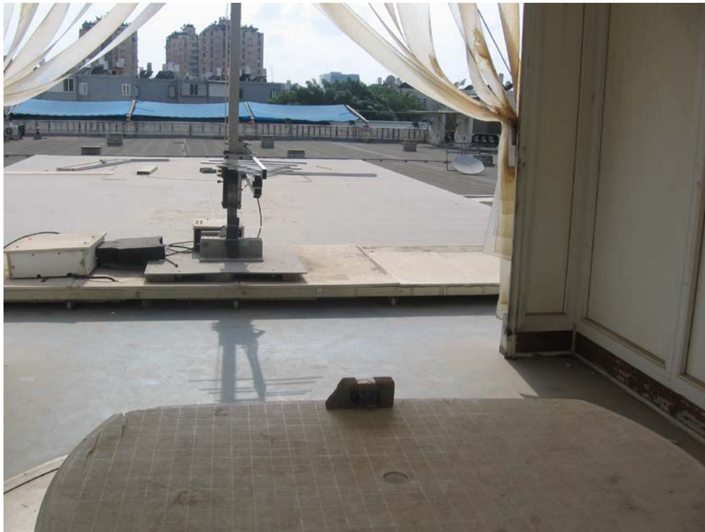
Figure 6. Radiated Emission Test, 200-1000MHz
