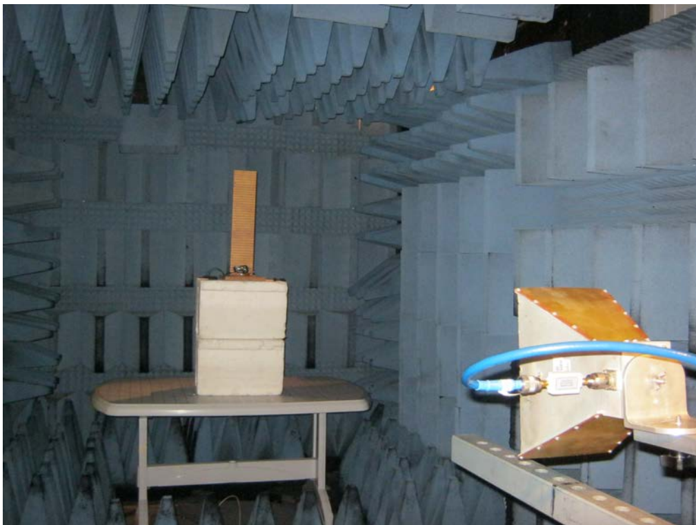
Figure 7. Radiated Emission Test, 1-18GHz
