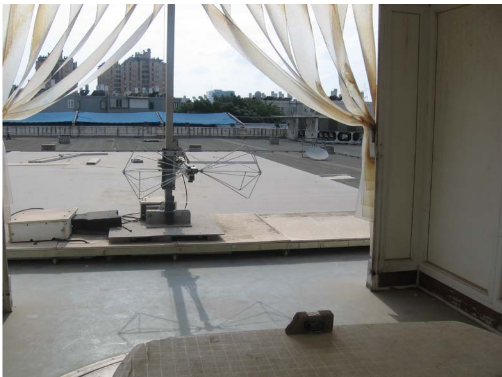
Figure 5. Radiated Emission Test, 30-200MHz
