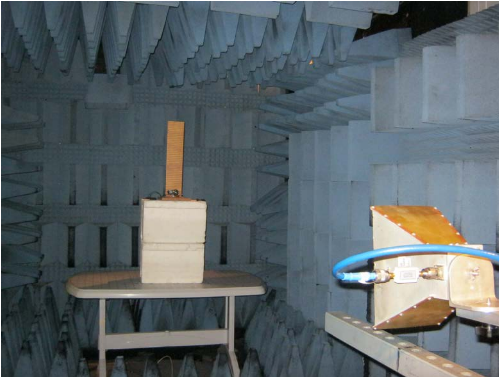
Figure 7. Radiated Emission Test, 1-18GHz
